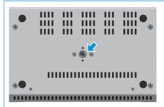
This is used when attaching the V-02HD MK II to a commercially available camera tripod. The socket is threaded for a 1/4" screw.
